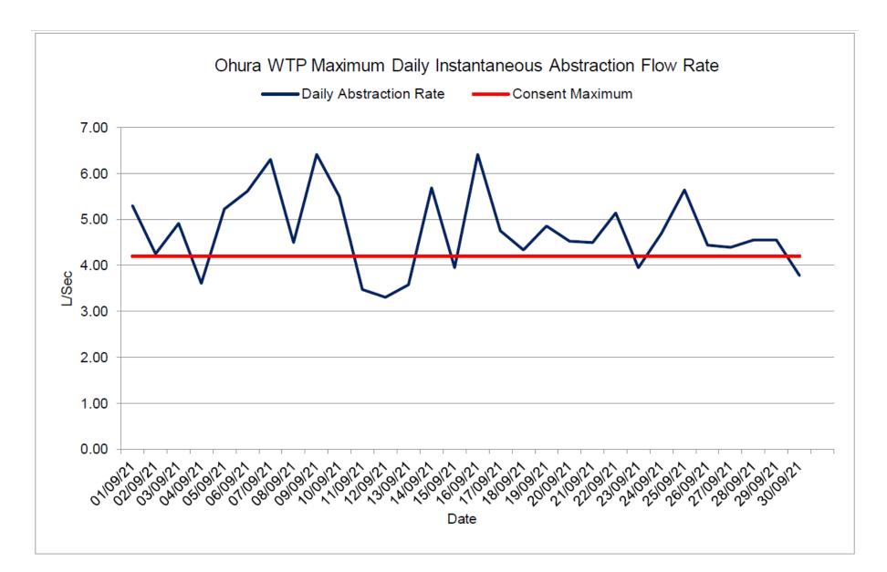
This shows the maximum abstraction rate in L/sec for each day. SCADA records minute data for flow in m<sup>3</sup>/hr then it is converted to litres/sec in excel. Even if the spike is for one minute then it will record as a failure.
